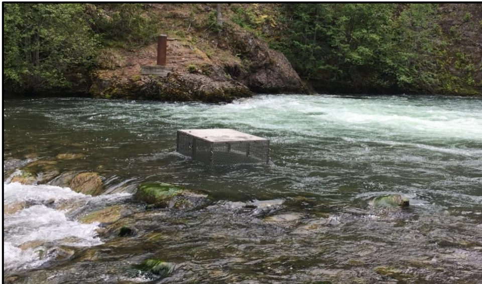
Figure 2. Stainless steel pen (0.9 m x 1.2 m x 1.8 m) used for holding Bull Trout after collection and before rapid response genetic testing and transport.
